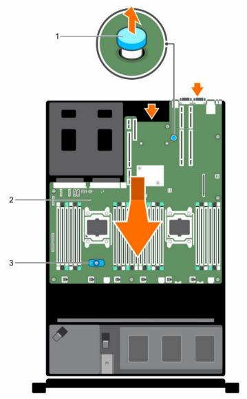
Figure 58. Removing and Installing the System Board
